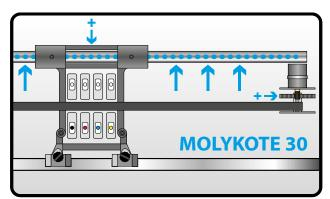
Pour alcohol (95% or higher) on a cloth and clean the carriage shaft thoroughly.
