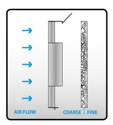
The fan filter collects the mist from the print head spray from the exhaust provided by the fan.
