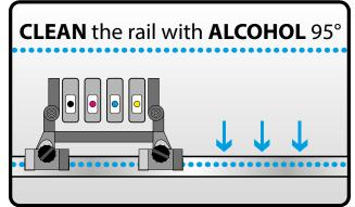
Unscrew the knob on the felt supports and remove them.
